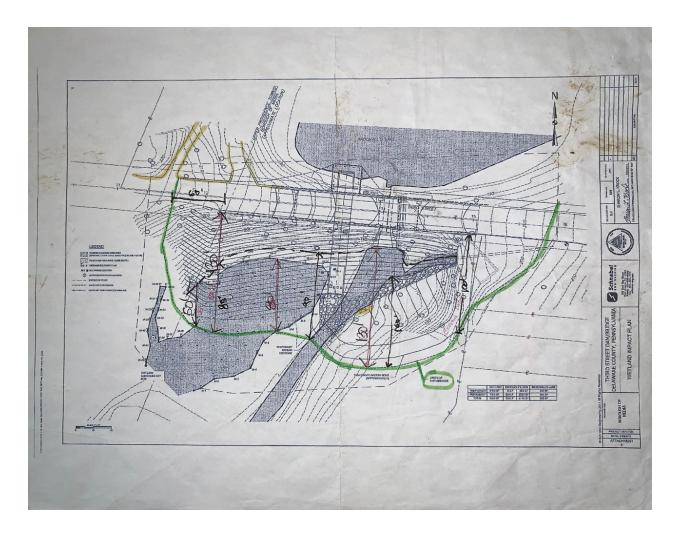
This is the Wetland Impact Plan by Sharon Krock of Schnabel Engineering, dated May 19, 2011. Our copy is complete with park mud! The green highlight covers the dashed line labeled "limits of disturbance," which we used as the boundary of the 1.1 acre disturbance area. The "existing path" is handwritten and the "temporary access road" is marked, both within that green line.
